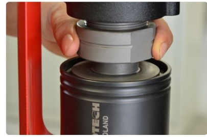
Tapping chuck feat. securing nut
